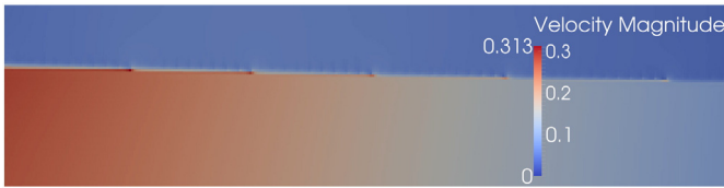
Fig. 5. Velocity field in the case of an a/d = 0.1 solitary wave during propagation, with a high velocity cell visible at the front face of the wave. Results obtained with Truchas.
