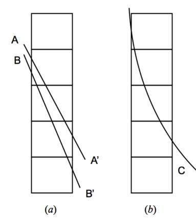
I) can only do so much: if the curvature us high, extending the height of the stencil doesn not help.
