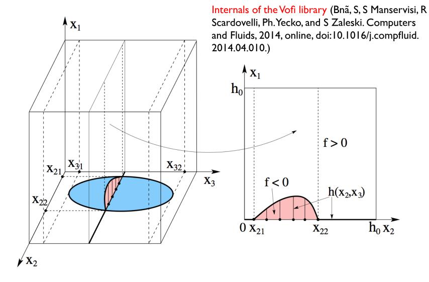
Figure 1: The cubic cell is subdivided in three right hexahedra after the computation of the two external limits of integration  $x_{31}$  and  $x_{32}$ , with the interface being present only in the central one (left); the internal integration requires the computation of the two internal limits of integration  $x_{21}$  and  $x_{22}$  and of the local height function h(right)
